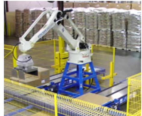
Figure 3. This palletizing robot is moving boxes. [Courtesy of Kawasaki Robotics (USA), Inc.]
