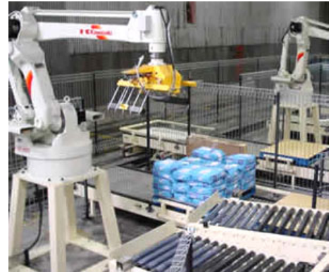
Figure 2. Palletizing is a common material handling application. [Courtesy of Kawasaki Robotics (USA), Inc.]
