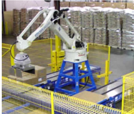
Figure 2. Palletizing is a type of material handling performed by robots. [Courtesy of Kawasaki Robotics (USA), Inc.]
