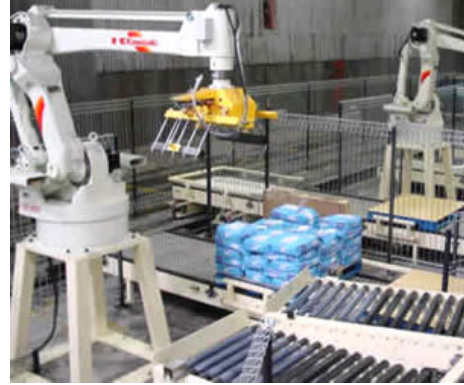
Figure 1. This palletizing robot can work for many hours without getting bored or tired. [Courtesy of Kawasaki Robotics (USA), Inc.]
