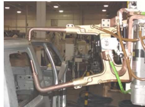
Figure 2. This spot welding gun would be difficult for a human to use. [Courtesy of Kawasaki Robotics (USA), Inc.]
