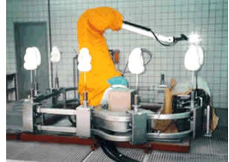
Figure 1. This painting robot can repeat a task many times with the same consistency. [Courtesy of Kawasaki Robotics (USA), Inc.]
