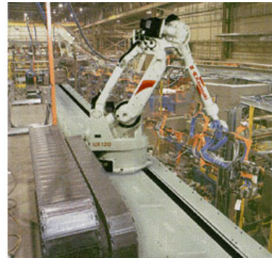
Figure 2. This toploader has a large range of movement. [Courtesy of Kawasaki Robotics (USA), Inc.]
