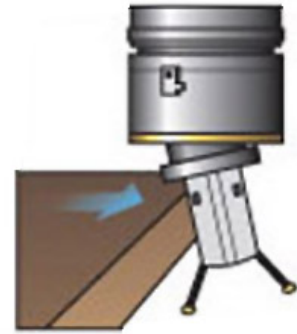
Figure 1. Collision sensors allow a robot to adjust its path if it makes contact with an object.
