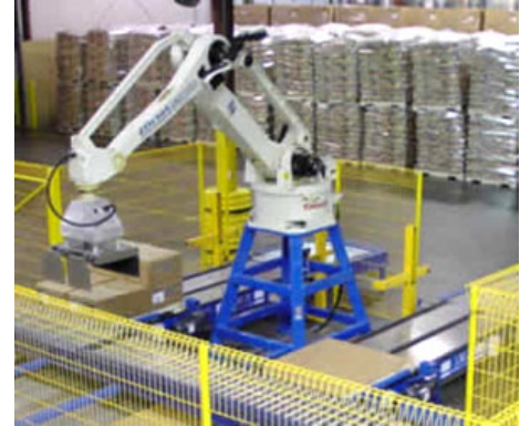
Figure 1. A palletizing robot. [Courtesy of Kawasaki Robotics (USA), Inc.]
