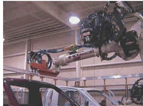
Figure 2. A spray painting robot. [Courtesy of Kawasaki Robotics (USA), Inc.]
