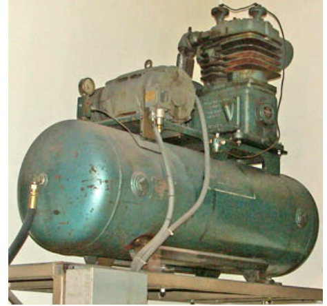
Figure 1. Pneumatic drives use a compressor to move air under pressure.
