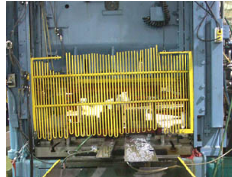
Figure 2. This guard can be adjusted for different sizes and shapes of materials.
