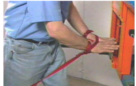
Figure 2. These wrist straps were developed to keep workers' hands from entering unsafe areas.
