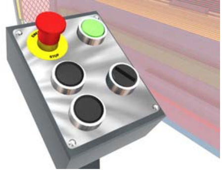
Figure 1. An E-stop switch brings a robot to an immediate, safe stop. (Courtesy of Banner Engineering.)
