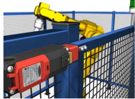
Figure 1. Interlocks cause a robot to stop when the gate is opened. (Courtesy of Banner Engineering.)
