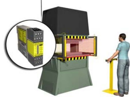
Figure 1. Two-hand controls require a worker to have both hands on the control before the robot starts. (Courtesy of Banner Engineering.)
