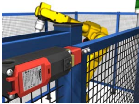
Figure 1. Use a barrier device like this interlock for robot safety. [Courtesy of Kawasaki Robotics (USA), Inc.]
