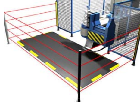
Figure 1. This presence-sensing mat causes the robot to stop when a worker stands on the mat. (Courtesy of Banner Engineering.)
