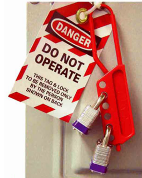
Figure 2. Workers must be trained to use safeguards such as lockout/tagout for robot safety.
