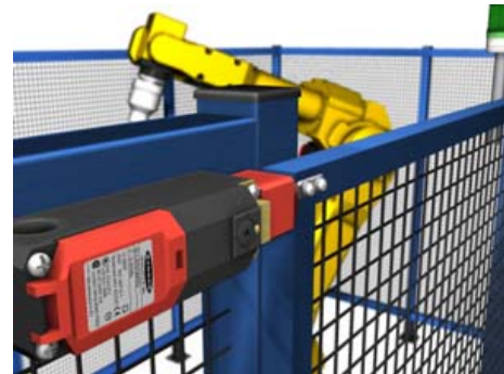
Figure 2. This interlock causes the robot to stop when the gate is opened. (Courtesy of Banner Engineering.)
